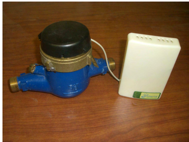
Pulse water meter wired to Wellspring BTU meter
